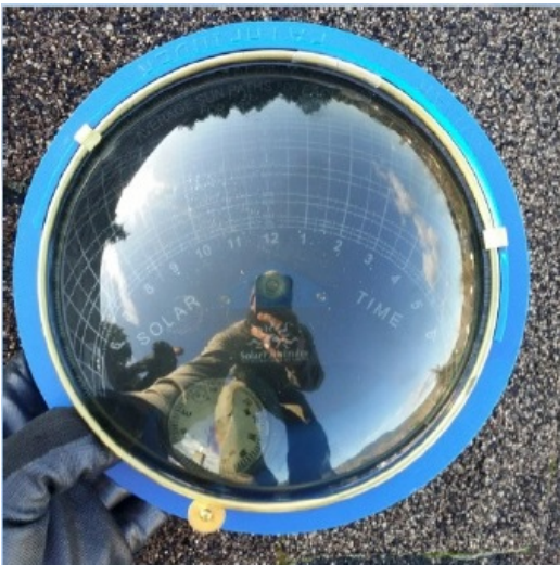
This Solar Path Finder is used in shading analyses to calculate the amount of energy that could be generated by solar panels at any given location.
