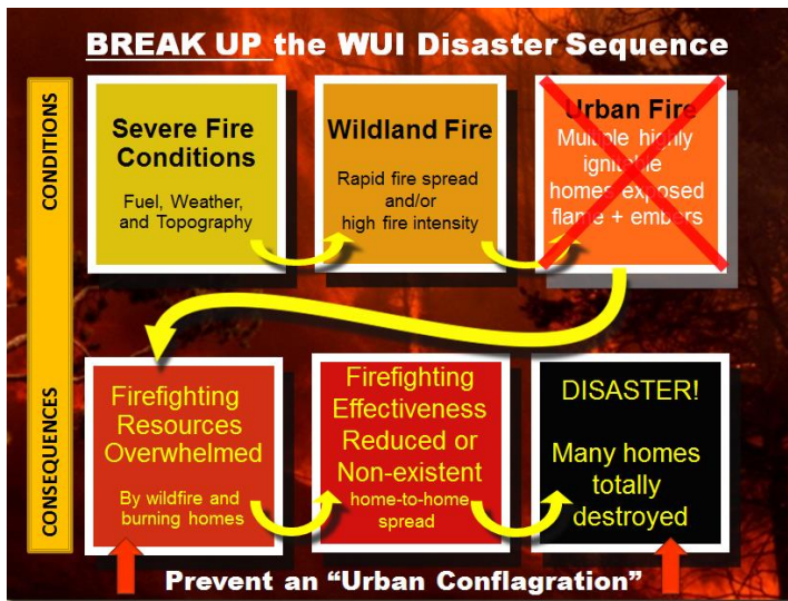
Figure 5. Wildland/urban interface disaster sequence. 75 It is possible to break up the disaster sequence by decreasing the number of highly ignitable homes exposed to embers, therefore reducing the number of homes ignited and removing the consequences of multiple structures lost.
