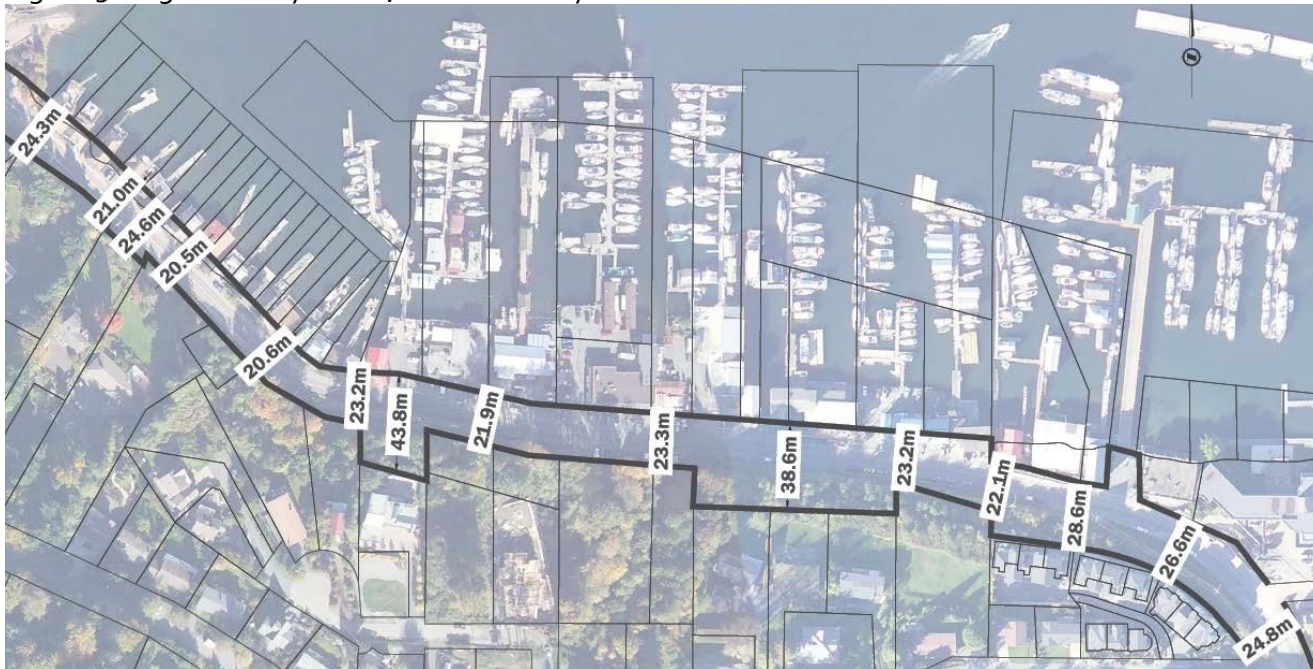
Figure 5. Right-of-way width, Cowichan Bay Road
