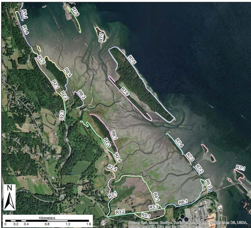
**Figure 21** Shoreline reaches for calculation of wave run-up
