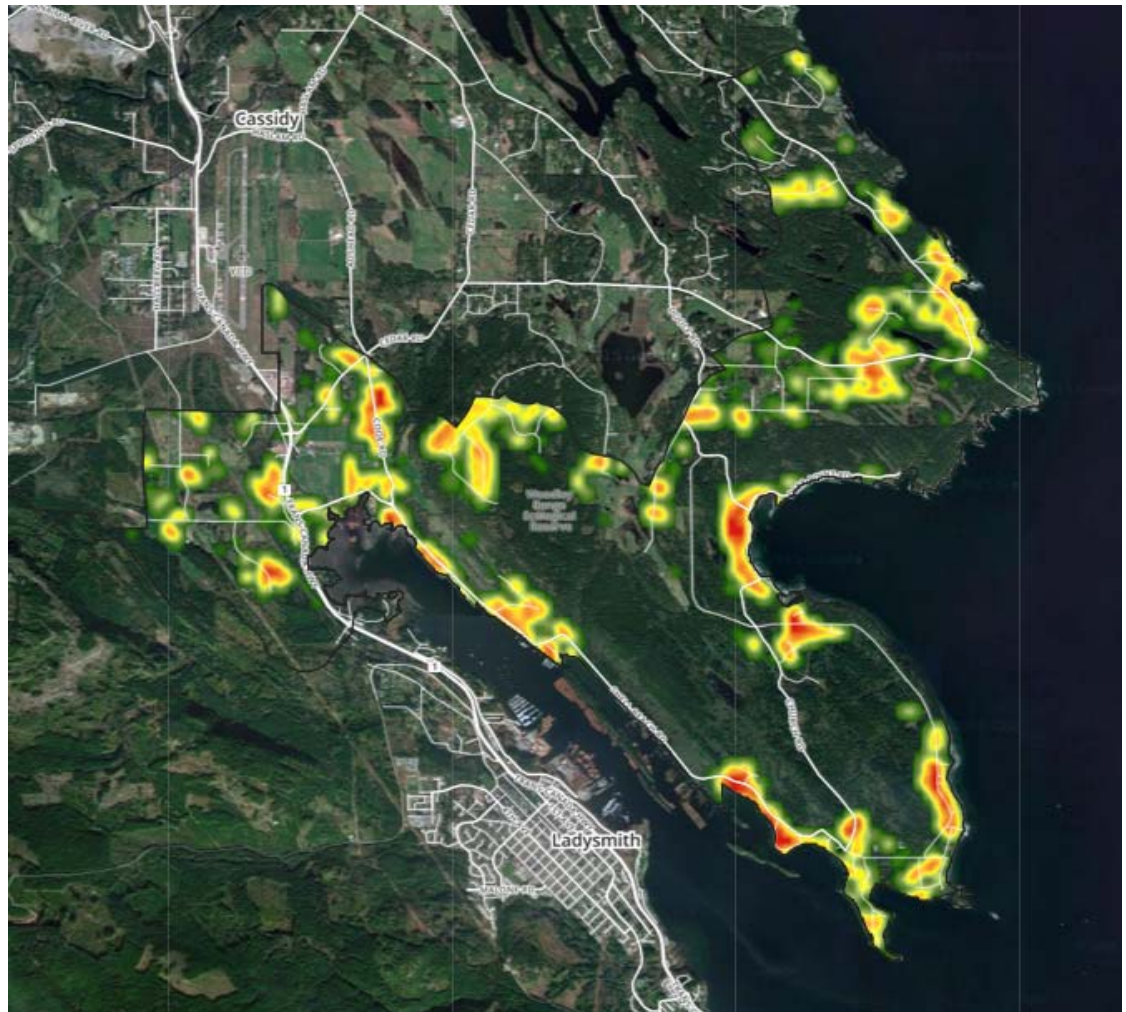
Figure 7-8. Areas of potential water-supply vulnerability based on increased demand and reduced recharge. Yellow-orange-red areas indicate zones of increased vulnerability.
