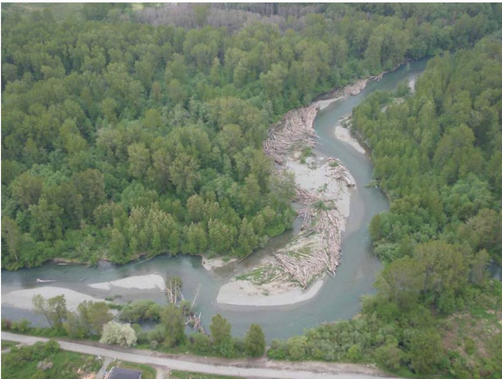
Photo A.1: Aerial view of the Cowichan River mainstem illustrating mid channel bars at km 4.3 and 4.5 where gravel and debris accumulate and intact riparian habitat extends over both left and right banks with Quamichan Road in the foreground (May 08).
